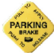
Figure 2-1 Parking brake knob
