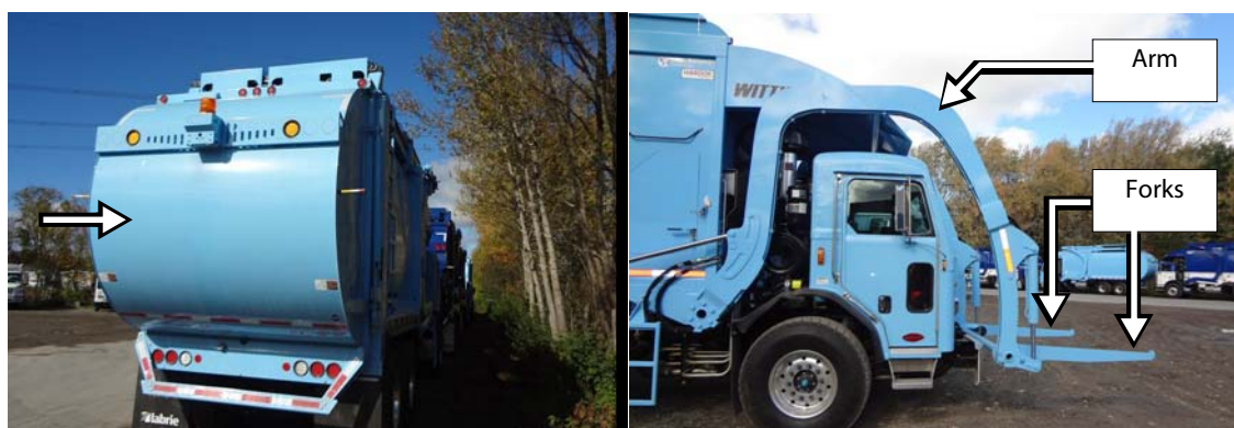
Figure 1-3 Tailgate (left), arms and forks (right)
