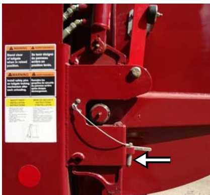
Figure 2-13 Tailgate safety pin in storage position
