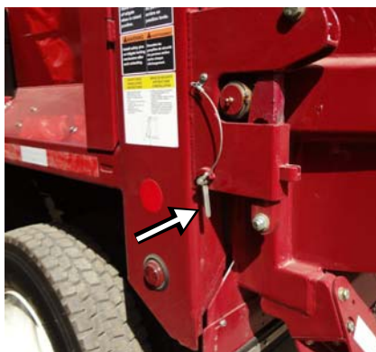
Figure 2-12 Tailgate safety pin in locking position
