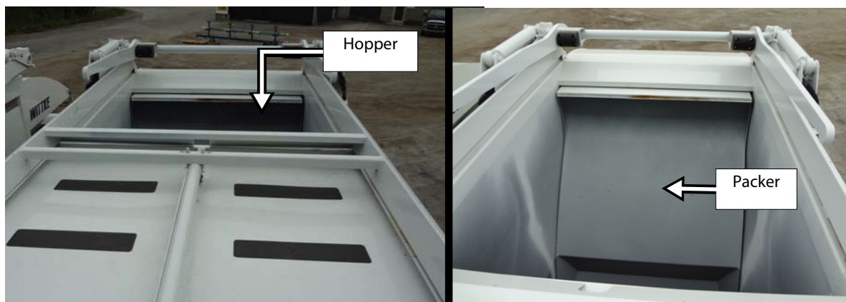
Figure 1-2 Hopper and packer
