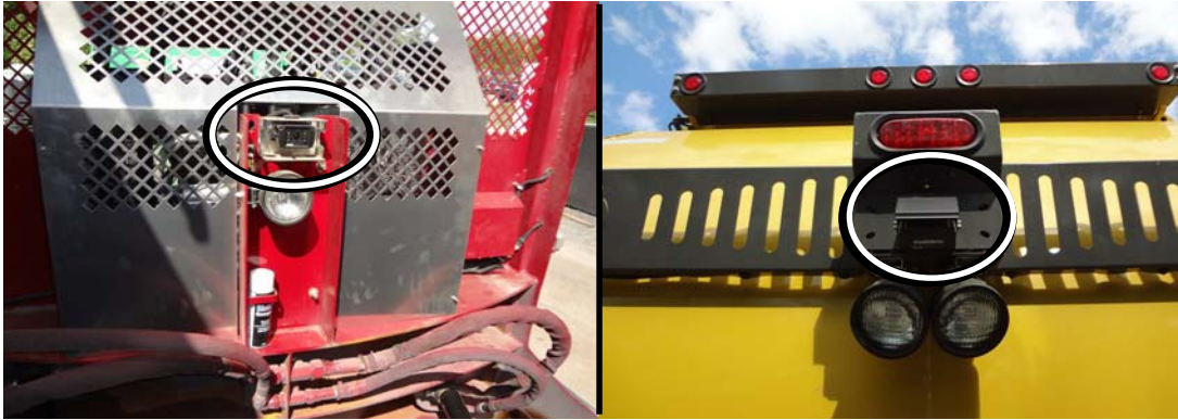
Figure 2-14 Camera inside hopper (left) and on tailgate (right)
