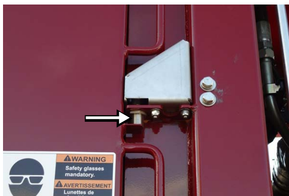
Figure 2-16 Side Access Door proximity switch
