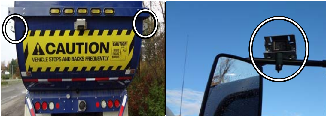
Figure 2-15 Cameras on both sides of tailgate (left) and on left-hand side mirror (right)
