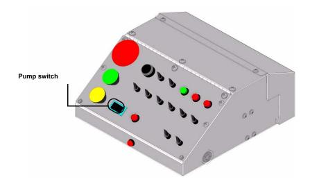
Figure 9. Pump switch on the console
