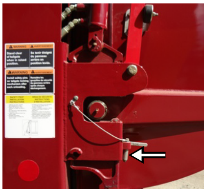
Figure 2-7 Tailgate safety pin in storage position
