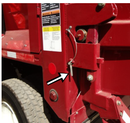
Figure 2-6 Tailgate safety pin in locking position
