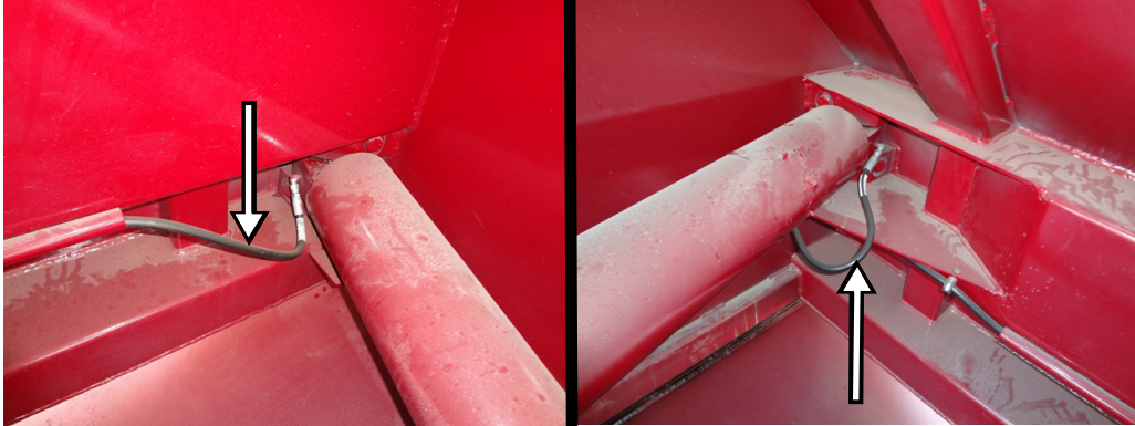
Figure 8-6 The optional grease fitting hoses is may be removed from the packer during this process.
