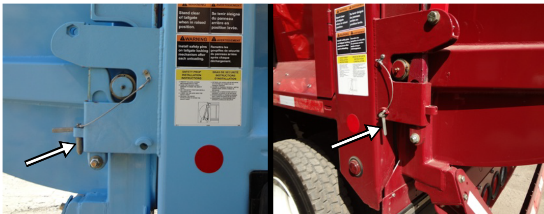
Figure 2-2 Safety pin (in storage position, left; in locking position, right)
