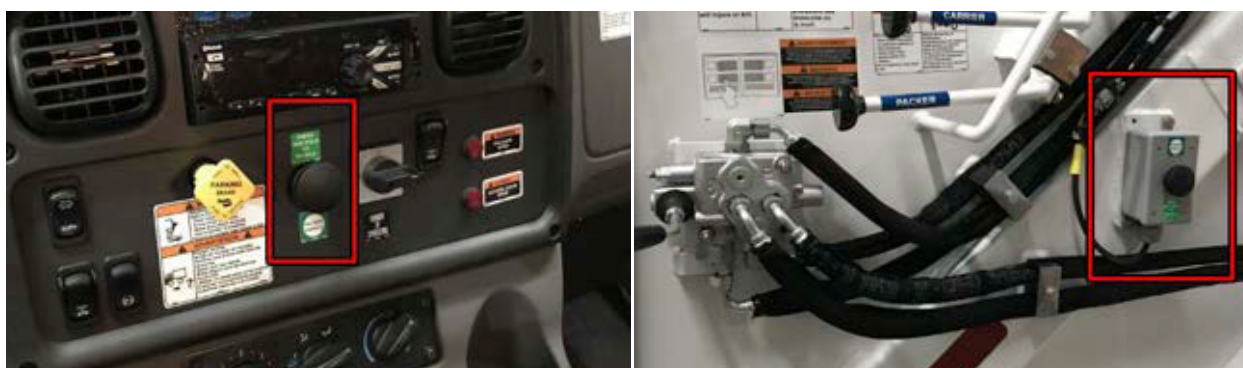
Figure 2-20 Driver enable button (left), Tailgate enable button (right)
