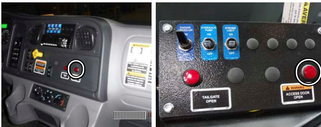
Figure 2-24 ACCESS DOOR OPEN light indicator (on dashboard, left, on optional console, right)
