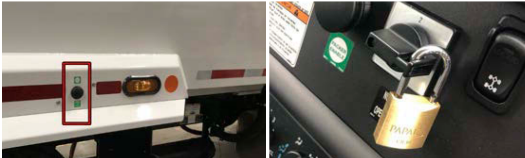
Figure 2-21 Mid-Body enable button (left), rotary switch (right)
