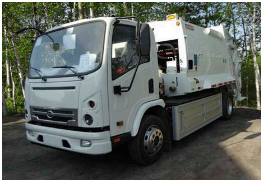
Figure 1-12 MINI REAR LOADER with electrically powered chassis
