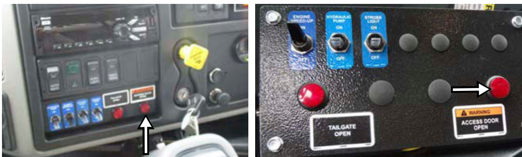
Figure 3-16 ACCESS DOOR OPEN Light (on dashboard, left, on optional console, right)
