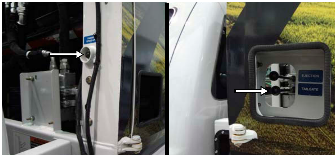
Figure 4-10 ENGINE SPEED-UP push-button (left), TAILGATE lever (right)
