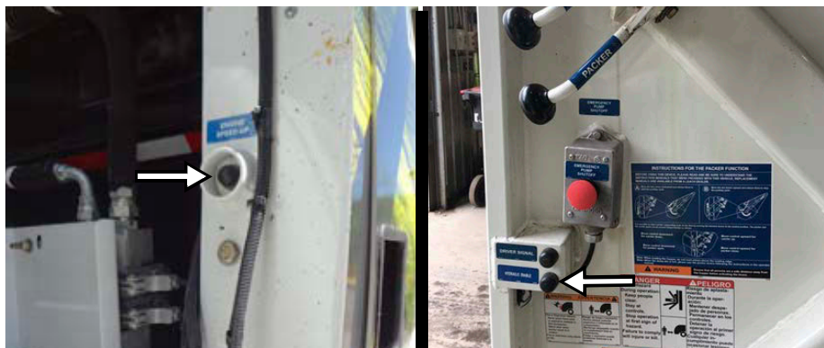
Figure 1-11 SPEED-UP buttons (HYDRAULIC ENABLE buttons on electrically powered units)
