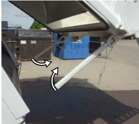
Figure 2-16 Putting back props into stored position
