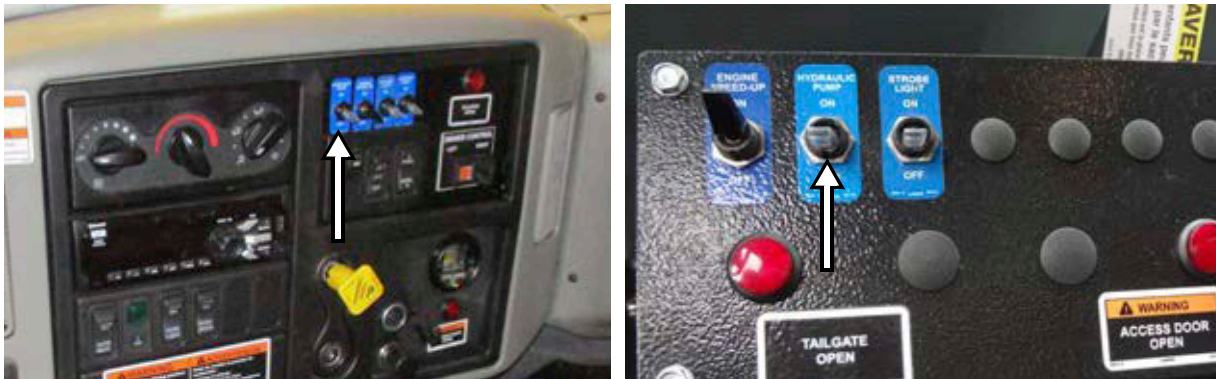
Figure 2-31 HYDRAULIC PUMP ON/OFF switch (on dashboard, left, on optional console, right)
