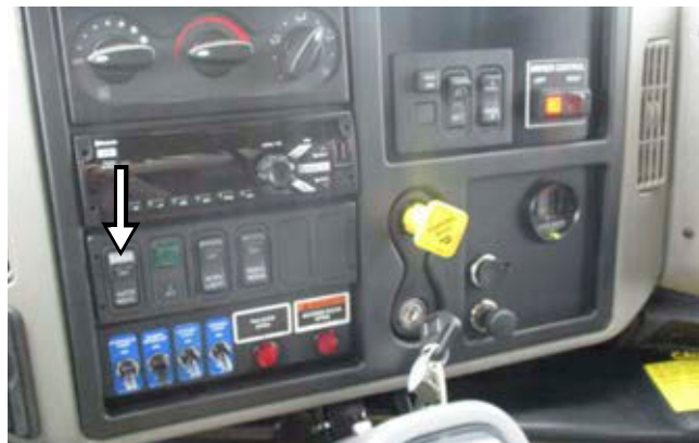
Figure 3-5 AUTO-NEUTRAL switch (on dashboard)
