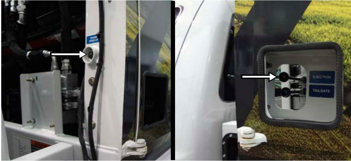
Figure 4-11 ENGINE SPEED-UP button (left), PUSHOUT lever (right)
