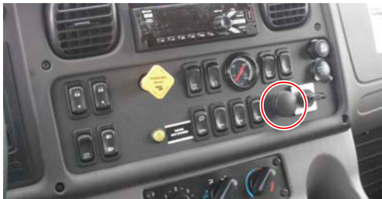
Figure 3-12 Driver enable button
