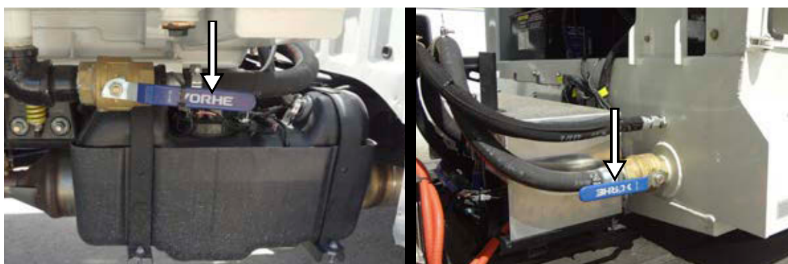
Figure 2-30 Suction line shut-off valve
