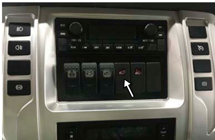
Figure 2-18 TAILGATE OPEN light indicator on dashboard
