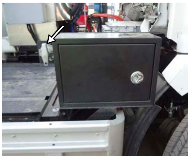
Figure 2-28 Master switch (on units w/ an electrically powered chassis)
