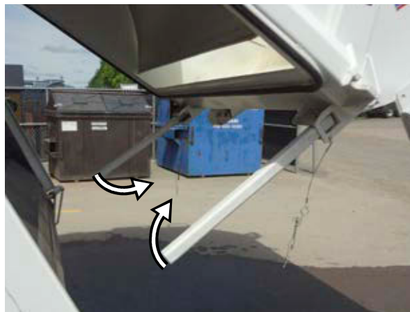
Figure 2-7 Putting back props into stored position
