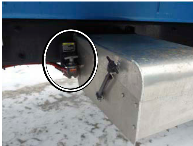
Figure 2-28 Master switch (on units w/ an electrically powered chassis)
