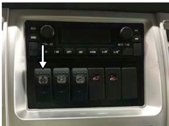
Figure 3-3 HYDRAULIC PUMP ON/OFF switch (optional switch/indicator layout)
