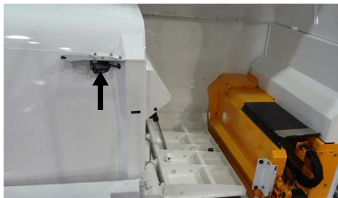
Figure 2-9 Camera on central RHS post
