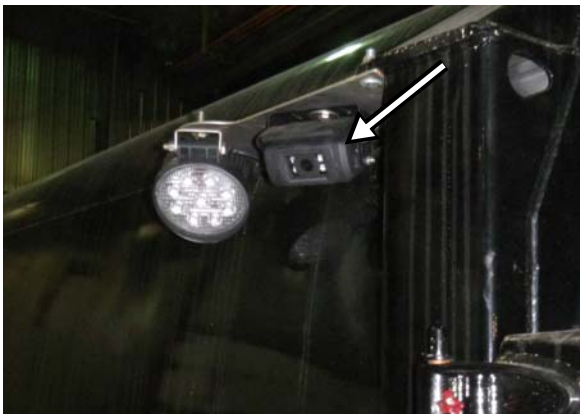
Figure 2-11 Camera on left-hand side mirror
