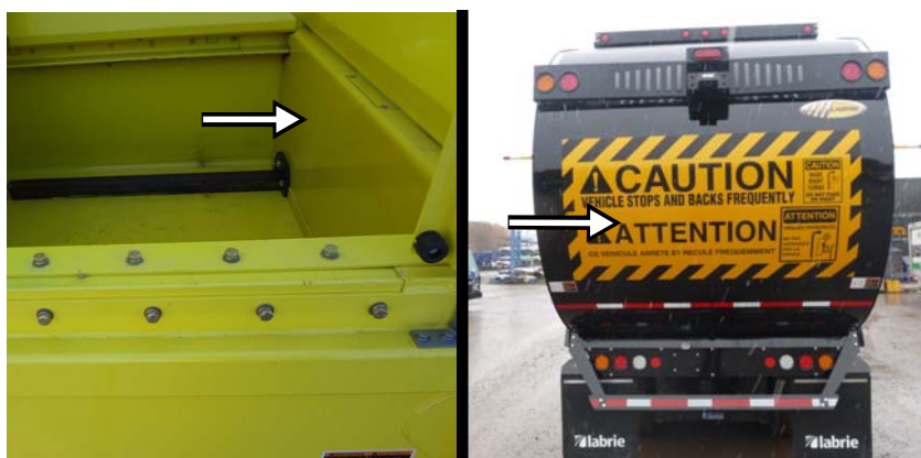
Figure 1-3 Packer panel (left); tailgate (right)
