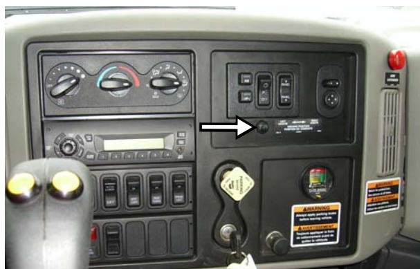
Figure 2-20 Driving position switch (optional)
