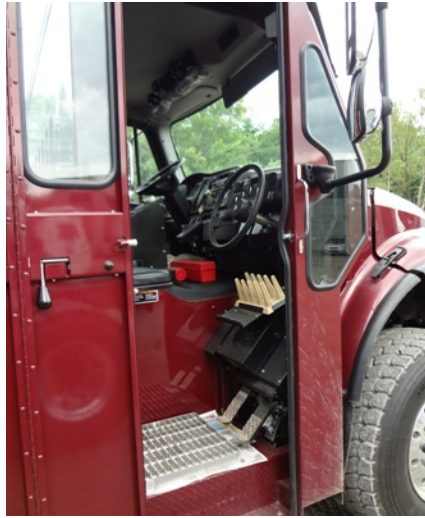
Figure 2-19 Right-hand side driving position installed by Labrie
