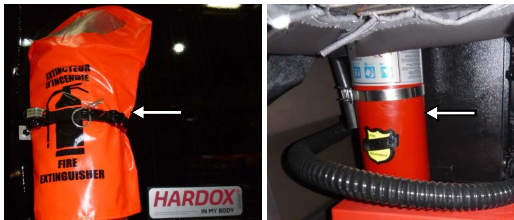
Figure 2-1 20-lb fire extinguisher (left); 5-lb fire extinguisher (right)
