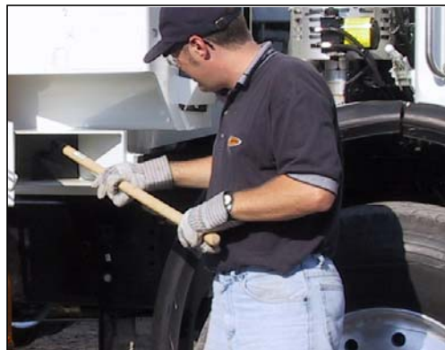
Figure 2-12 Removing debris through the clean-out trap
