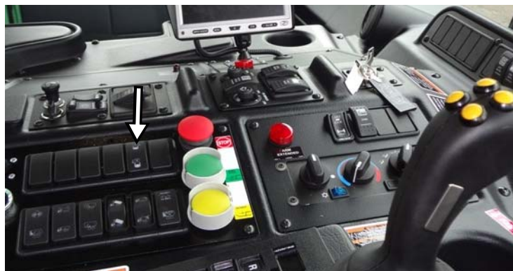
Figure 2-21 Joystick selector switch (optional)
