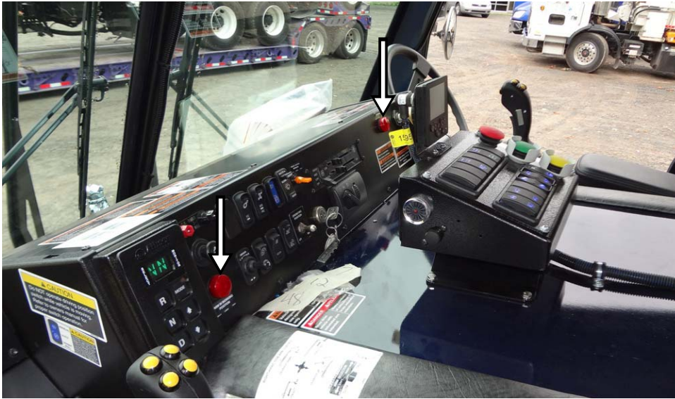
Figure 3-29 Arm Extended warning lights
