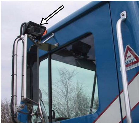
Figure 2-11 Camera on left-hand side mirror
