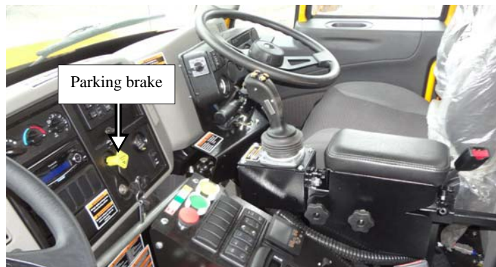
Figure 2-19 Right-hand side driving position installed by Labrie
