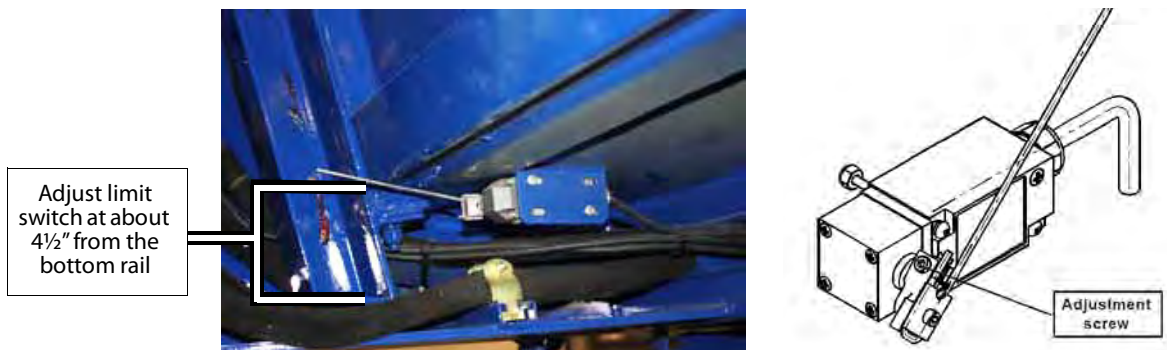
Figure 5-12 Bucket limit switch
