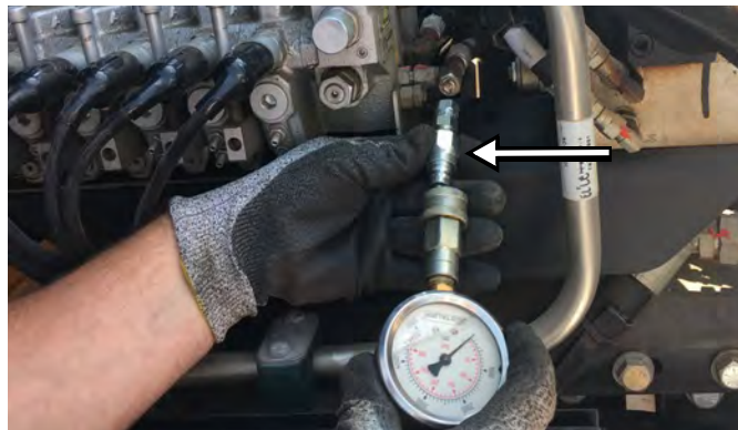
Figure 6-8 Connecting the gauge to the test port using an adaptor
