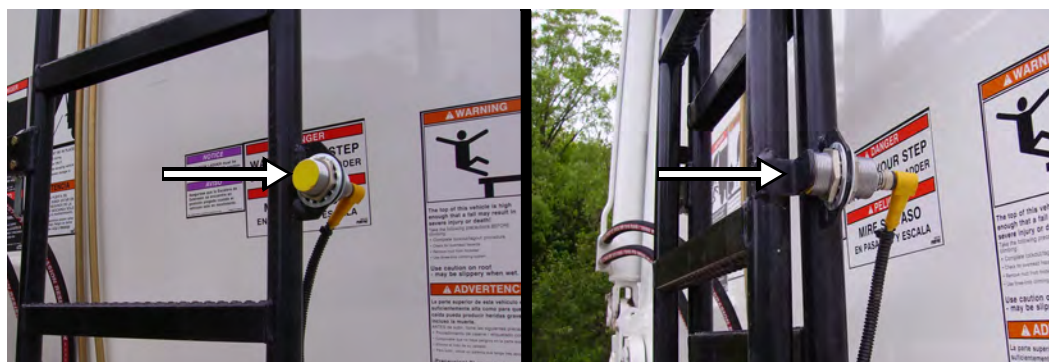
Figure 2-4 Extension Ladder proximity switch with ladder deployed (left) and in stored position (right)
