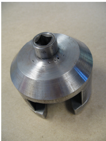
Part Number 153011 Shutoff Valve Removal Tool
