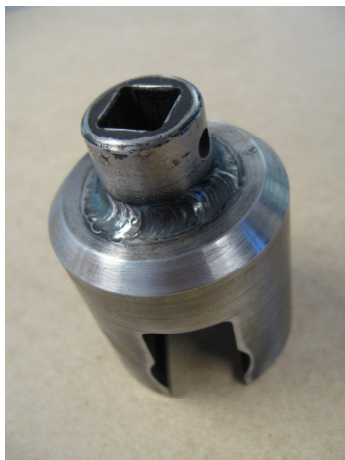
Part Number 153110 Vent Valve Removal Tool
