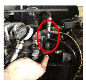
• Start the engine, engage the pump and operate each circuit, holding the control after it reaches it travel limit, and note the pressure.
