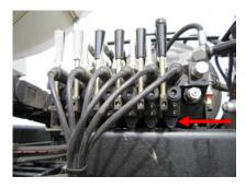
• Remove the o-ring cap plug.
