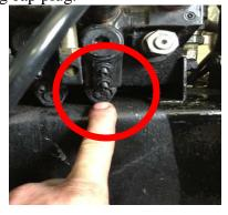
• Turn the internal adjustment screw with an Allen wrench clockwise (in) to increase pressure, or counter-clockwise (out) to decrease pressure.
