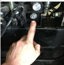
O Using an Allen wrench, hold the adjustment screw and loosen the adjustment screw jam nut with an open-end wrench, by turning the nut counter-clockwise (out).
