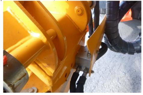
Labrie updated the holding valve to a version that integrates a flow divider to provide smooth and even operation of both grabbers. The flow divider function is preset at the factory; adjustment is not necessary or possible. The grabber holding valve is adjustable; checkout and adjustment information is attached.
