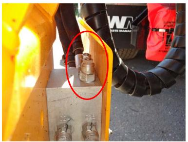
1. Remove the dust cap on the pressure test port of the arm directional control valve and attach a 0 - 3,000 PSI pressure gauge into the pressure test port.
