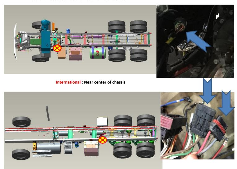
Crane Carrier (CCC): Rear of transmission, on the right side
