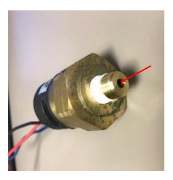
Next, locate the hole on the back of the pressure switch. Using a 3/32" hex wrench, remove the long, threaded needle and clean the adjustment port with electrical contact cleaner.
