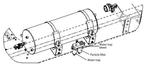
Bleed all the water from the water trap and the air filter bowl located on the chassis to helps keep residual moisture out of the body air system.
