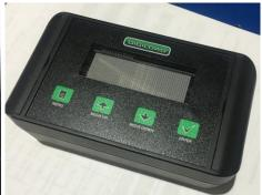
To flush the memory, just connect a standard USB key with 16Mb memory or more, and the transfer is automatic. (Transfer data to USB Key + Flush module memory).
