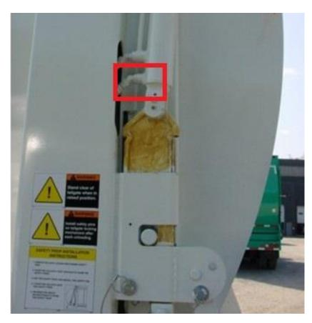
We have identified that there are two different versions of the p/n-10384 orifice fittings that vary in seating depth. Either dimensional orifice will work in standard TG cylinder HYC00320-04, however, only the shorter version of the orifice fitting will work in tailgate cylinder HYC00323, which is a heavier duty cylinder used on CNG powered units.
