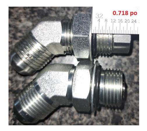
If you have the HD tailgate cylinder HYC00323 installed, and it is leaking out of the case end orifice fitting it is likely that the longer version of orifice p/n-10384 was installed. To rectify the issue, replace p/n-10384 orifice with orifice fitting p/n- HYF05120 and #08 JIC fitting p/n 217102.
